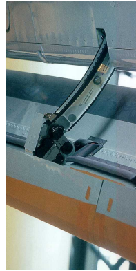
Fig. 28 Mounted Slat track for AIRBUS A320
