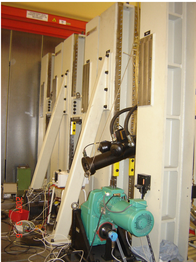
Fig. 32 Test rig of ASCO at the VUB (Free University of Brussels). In the foreground, a bi-axial test rig can be seen.
