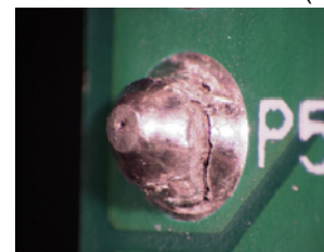
Figure 9 Example Solder Joint Crack
