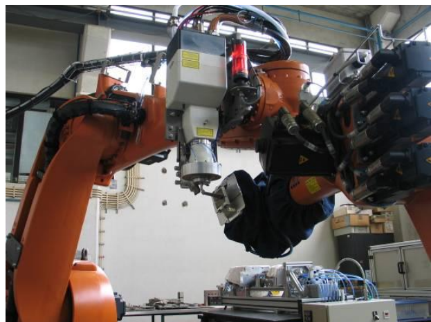
Picture 13 Robotic cells for laser welding at ISQ. Two different strategies were tested: First to have the part fixed in a cradle and moving the robot only and secondly moving the part coordinated with the movement of the welding robot.
