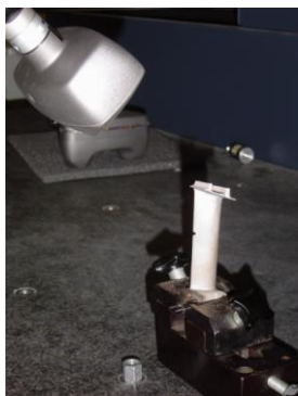
Picture 6 Laser scanner scanning a turbine blade
