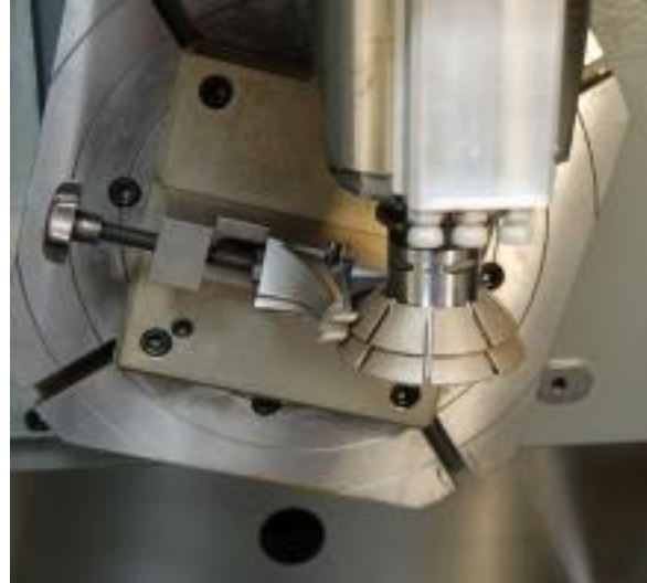
Picture 17 Machining of the z-shaped interlocks, another challenging task. The interlocks can only be milled and grinded with highly specialised tooling and require a high working effort.
