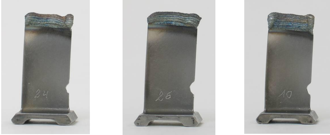
Picture 14 Some welding results during the second period. Especially the leading and the trailing edge points were a challenging task to be solved. In the course of trials, the results improved significantly.
