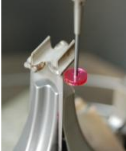
Picture 16 Touch-trigger-probing, a form of high accuracy tactile measurement, of characteristic points to check for the part's positioning
