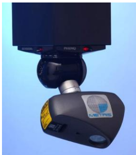
Picture 5 A typical laser scanner as used for incoming inspection. Line scanners of this type like the one showed deliver a point cloud (meshed data STL)
