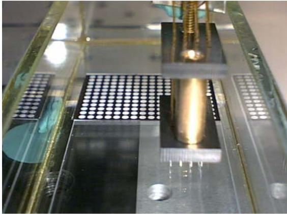
Figure 7. Photograph showing a 16-channel matrix “print head”, as well as microarray substrate and sample chambers.
