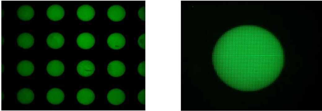
Figure 4. Fluorescence images of poly-L-lysine patterns (defined by lithography). Each area has a diameter of  $180\mu\text{m}$  and fulfilled or half filled of dot arrays of  $2\mu\text{m}$  diameter and  $4\mu\text{m}$  period.
