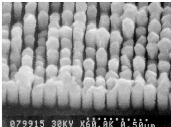
**Figure 2.** Scanning electron micrograph of nano-dot arrays formed by electroplating, defined by nanoimprint lithography.
