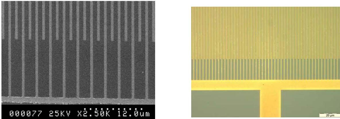
**Figure 8.** Photomicrography (right) sub micrometer inter-digital electrode of gold on a glass substrate, and (left) enlargement, showing 0.15 $\mu\text{m}$  line and 0.95 $\mu\text{m}$  spacing features.
