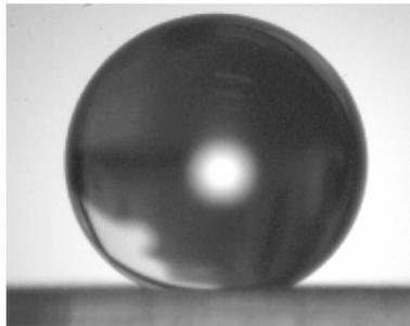
Figure 5. Microphotograph of a water droplet on patterned hydrophobic surface of a pillar array of height  $10\mu\text{m}$  and a period of  $10\mu\text{m}$ , showing a contact angle larger than  $150^\circ$  and super hydrophobic wetting properties.
