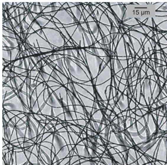
**Figure 3:** Photograph of long magnetic nanowires made by submitting a mixture of magnetic particles to a 25 mT magnetic field during 5 min. The chains are bent by gravity after field removal.
