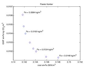
Pareto frontier for the multi-objective optimisation example: the upper point is for all weight to cost objective function while lower/right is for all weight to environmental objective function.
