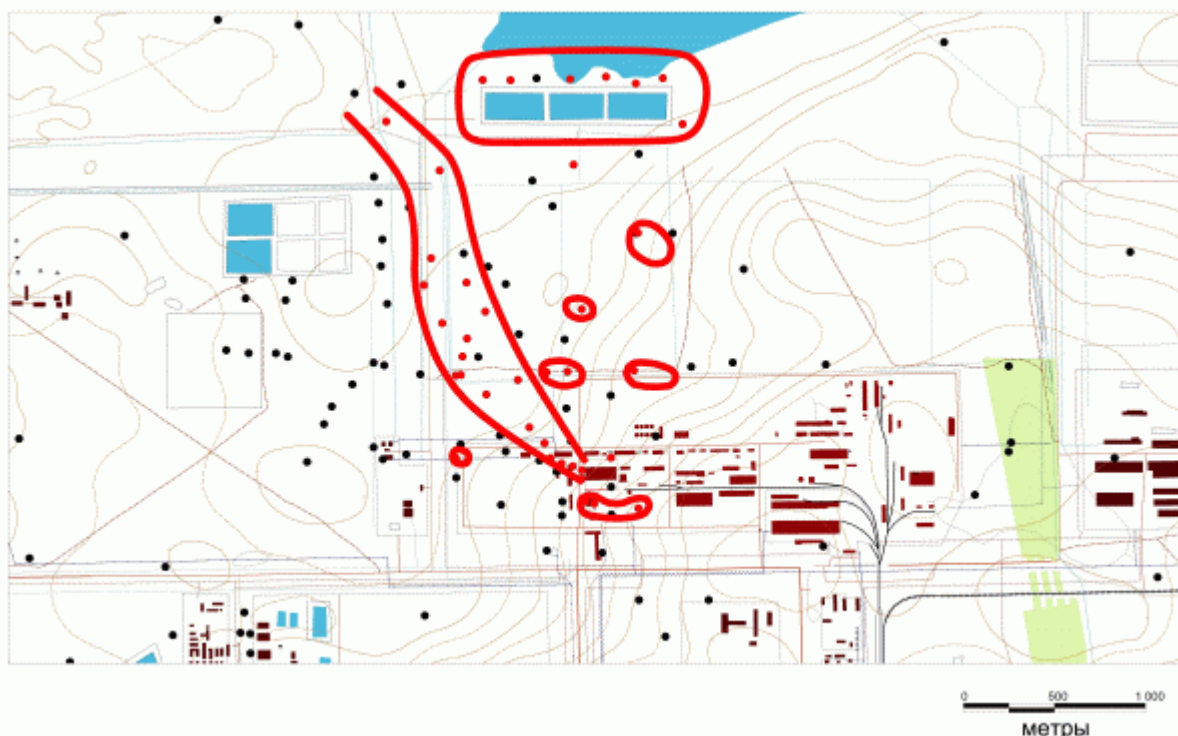
Fig.8. Hotspots of groundwater contamination with mercury above 500 ng/l according to 2002 investigation of observation boreholes
