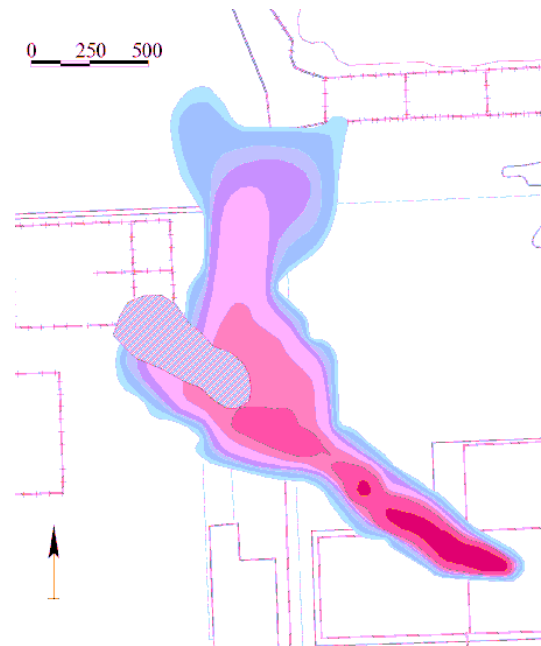
Fig.10. Spread (m) of plume of groundwater mercury contamination on the results of simulation of hydro-geological conditions as of 2031 (third prognosis scenario)
