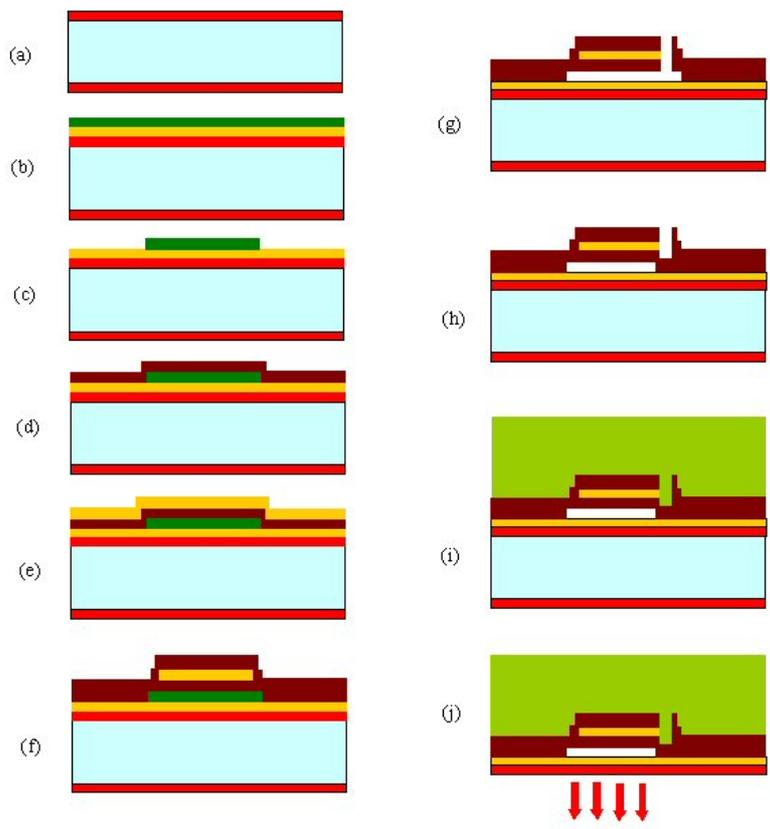
Fig. 1 Steps of the fabrication of a cMUT, using the “Reverse Fabrication Process”.
