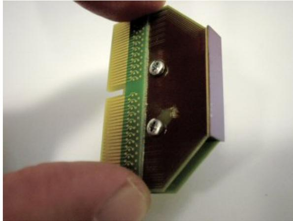
Fig. 2 cMUT transducer soldered to a rigid PCB circuit
