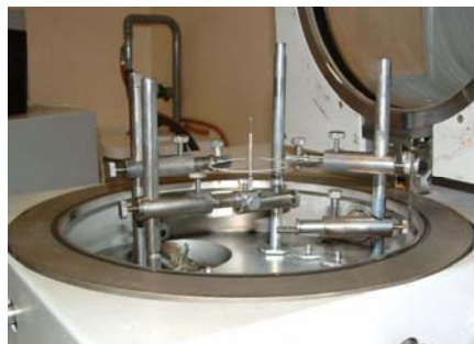
Fig. IV.3 Evaporation chamber and coating equipment developed at the University of Tartu
