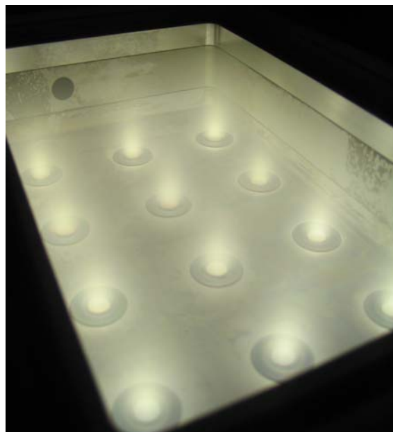
Oblique view of an oxygen plasma ( P = 1200\text{ W} , p_{O_2} = 19\text{ Pa} )
