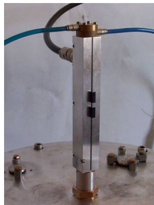
View of an elementary plasma source implemented on the top flange of the cylindrical chamber
