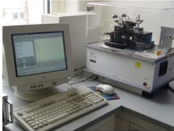
Ball on disc test apparatus
