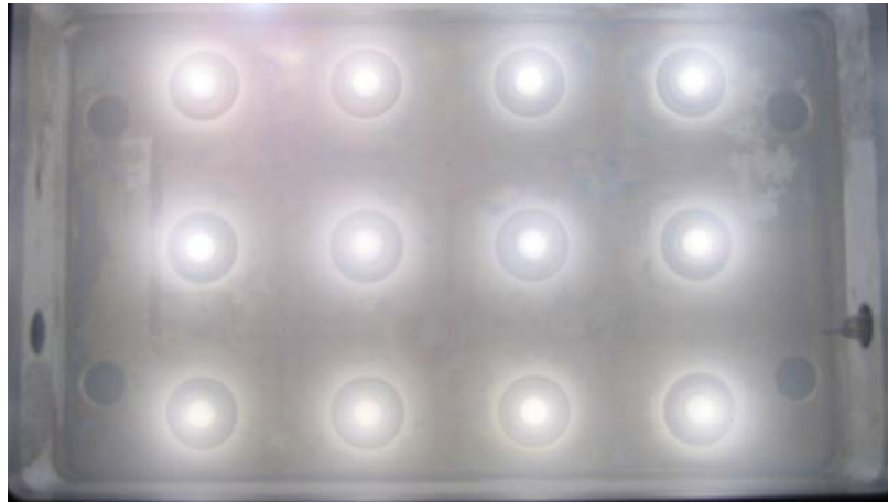
Top view of an oxygen plasma ( P = 1950\text{ W} , p_{O_2} = 7\text{ Pa} .)
