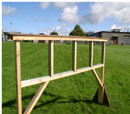
Fig. 2: Unsheltered exposition racks in the UK test site.
