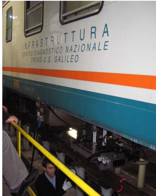
U-Rail inspection unit as installed under the rail vehicle “Galileo” provided by RFI
