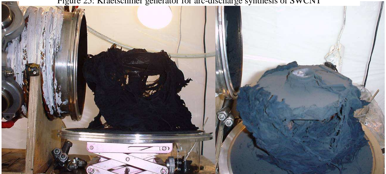
Figure 26: Nanotubes produced by arc-discharge at YANGTZE.
