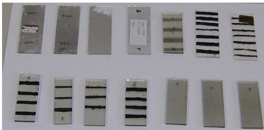
Figure 27: Samples of carbon nanotube networks and painted leads on glass and FTO coated glass prepared for testing on solar energy systems.
