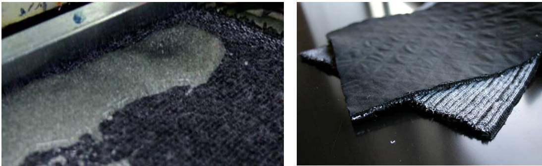
Figure 5: Safe&Cool water binding polymer on fabric layer: Racla coating (left image) and quilted membrane retaining water binding polymer (right image)
