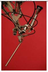
Figure 5: PICO Endoscope with exoscope camera mounted on motor driven adjustment unit
