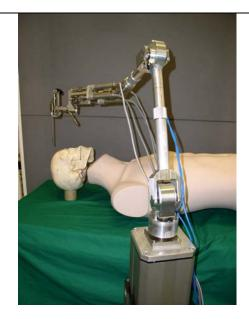
Figure 1: PICO Demonstrator hardware (stand, drives, endoscopes)
