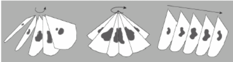
Figure: Fan-scan, rotational scan and translational scan
