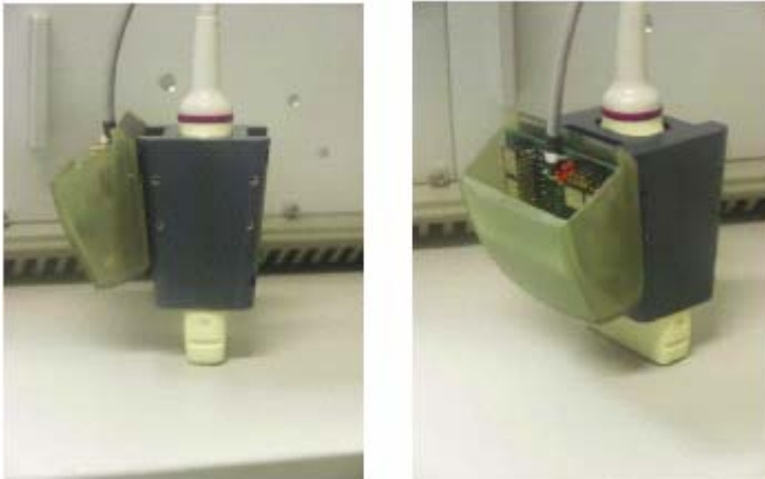
First generation functional model for fan scan freehand use
