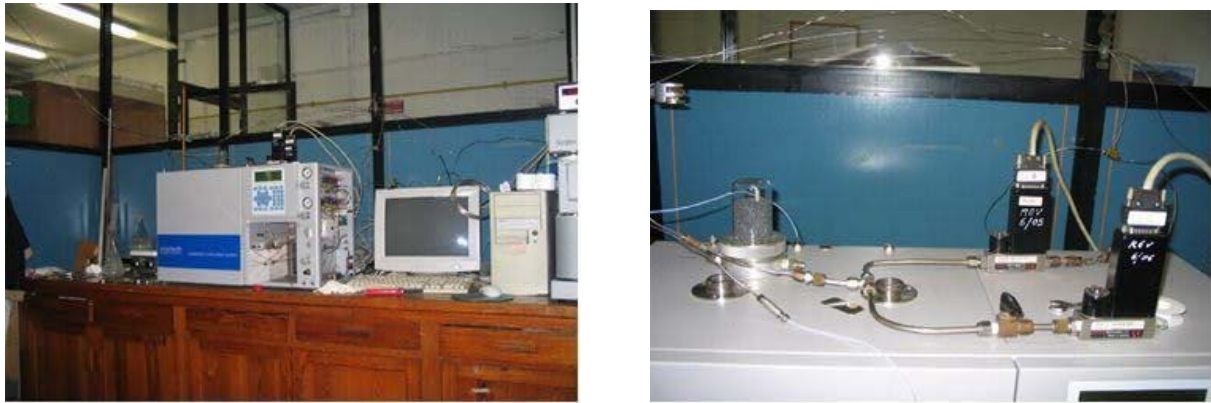
Fig. 25: ECS 4010 - Global View and Mass Flow Controllers for Mixture Preparation.
