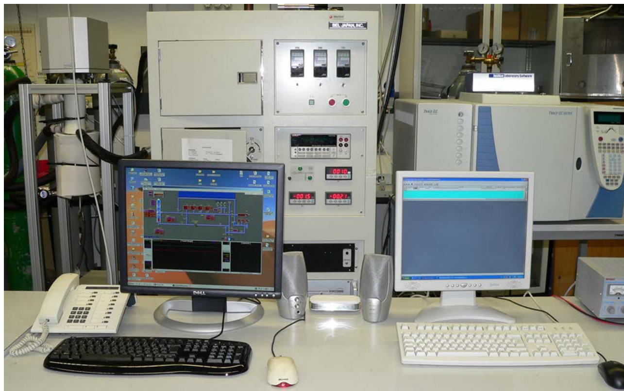
Fig. 9: Picture of the apparatus for multi gas sorption measuring in circulating quasi steady atmospheres
