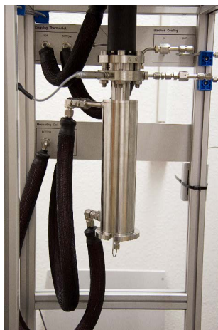
Fig. 13: Different Measuring cells and thermostating devices for the new ISOSORP Mono Gas HP-flow
