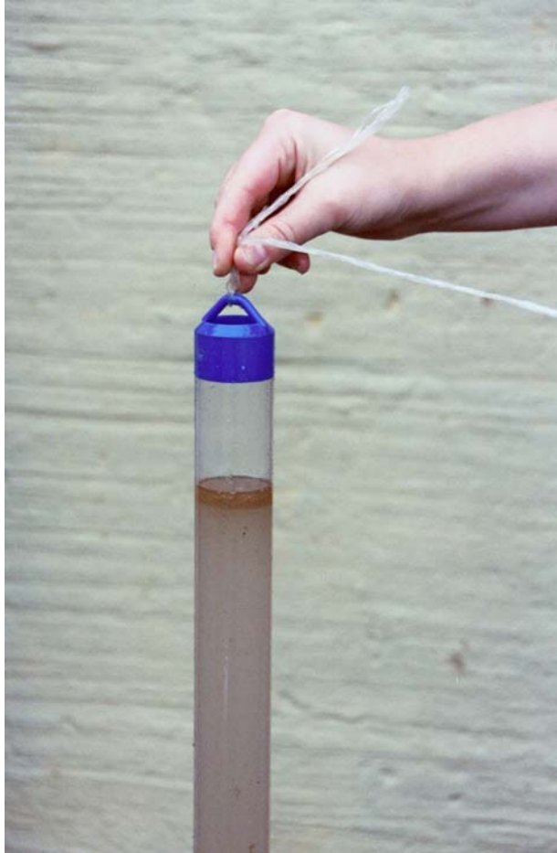
Figure 4: Groundwater with oil layer
