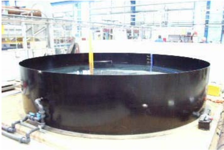
Figure 1: Test Tank with pumping system to control fill level.
