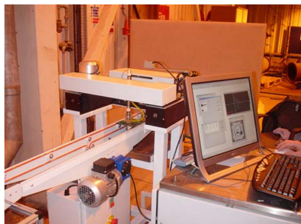
Figure 10: SAM Scanner incorporating PCB conveyor system.
