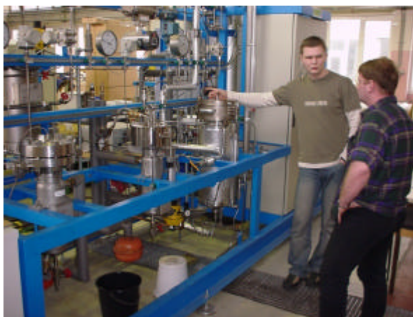
Fig. 16: Pilot plant for the precipitation of the polyphenols by supercritical CO 2 ; picture taken at NATEX Prozesstechnologie GesmbH (Ternitz, Austria)
