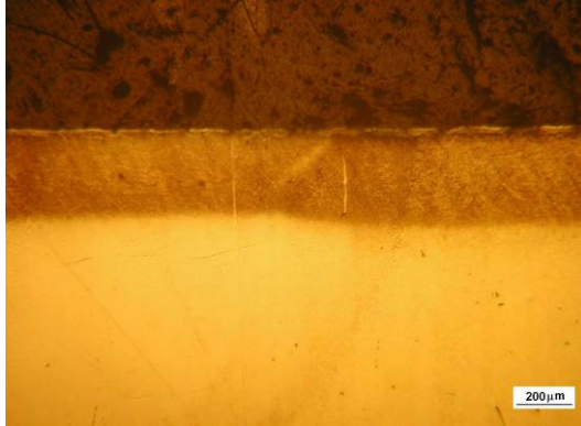
Figure 25: Transition between the alloyed and non-alloyed areas for steel 1.2365 laser alloyed with WC-Co
