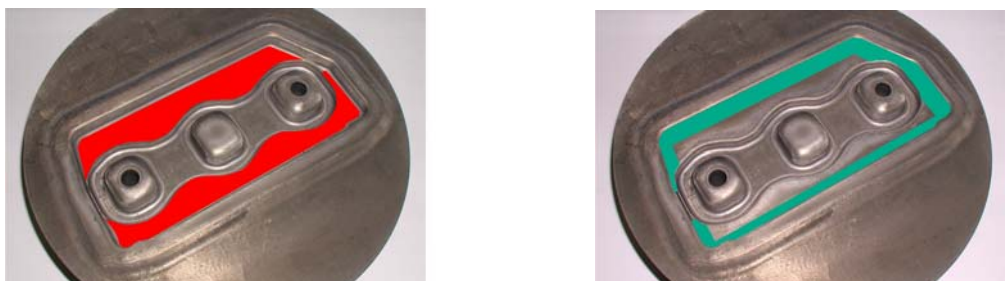
Figure 38: Laser dispersed areas of the Mould "MTK" – Left side: area of the 1st mould, right side: reduced area of the 2nd mould
