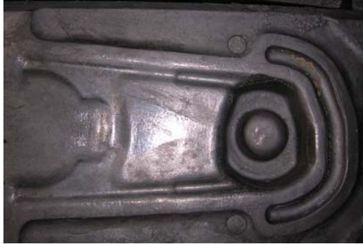
Figure 79: Applied lower part of the 1st Mould "BENE" (after 3rd polishing)
