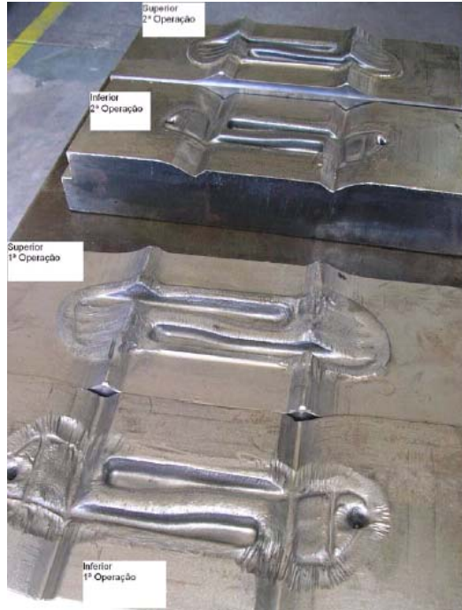
Figure 75: Applied 1st Mould "FAF" (fig., front) and 2nd Mould "FAF" before its application (fig., back)
