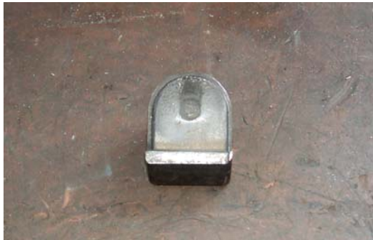
Figure 74: Mould "DMF" after 5.000 die casting cycles
