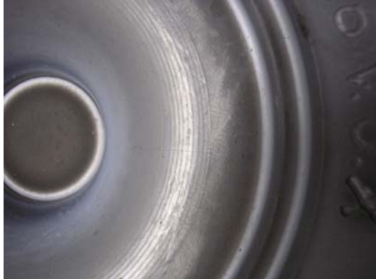
Figure 44: Surface of the Die "RAS" with one crack
