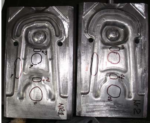
Figure 57: Die "BENE" (upper and lower part) provided for testing the combined treatment
