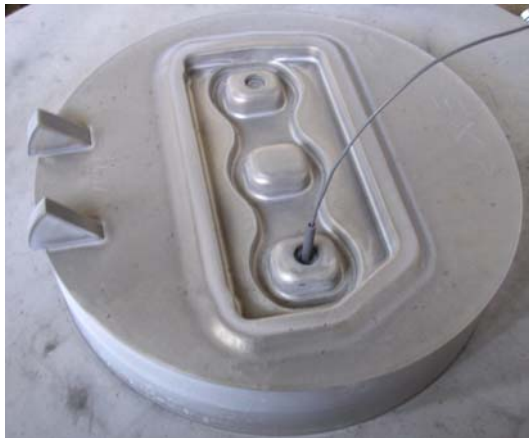
Figure 51: Die "MTK" after plasma nitriding
