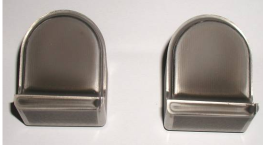
Figure 62: Dies "DMF" after plasma nitriding
