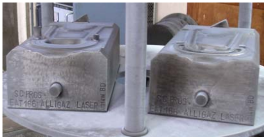
Figure 58: Die "BENE" after plasma nitriding
