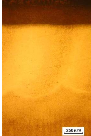
Figure 82: Micrograph of a part made of steel 1.2344, treated by laser dispersing and plasma nitriding
