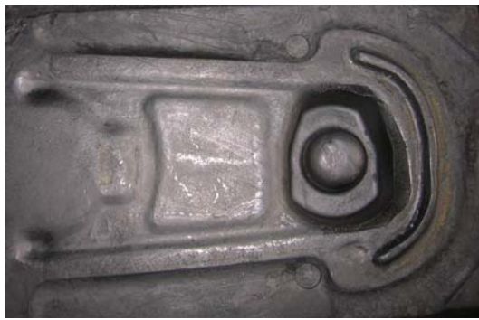
Figure 80: Applied upper part of the 1st Mould "BENE" (after 3rd polishing)
