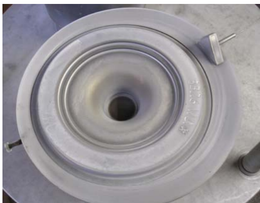
Figure 43: Surface of the Die "RAS" without cracks
