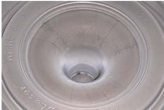
Figure 36: Formed cracks – 1st Mould "RAS"
