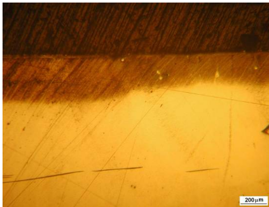
Figure 26: Transition between the dispersed and non-dispersed areas for steel 1.2365 laser dispersed with TiC
