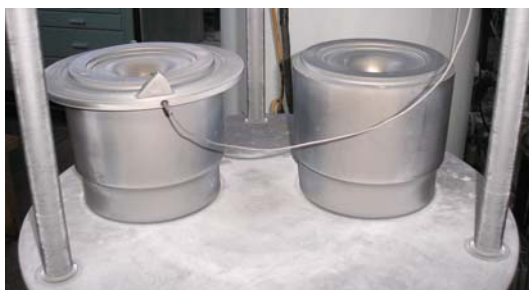
Figure 42: Dies "RAS" after plasma nitriding
