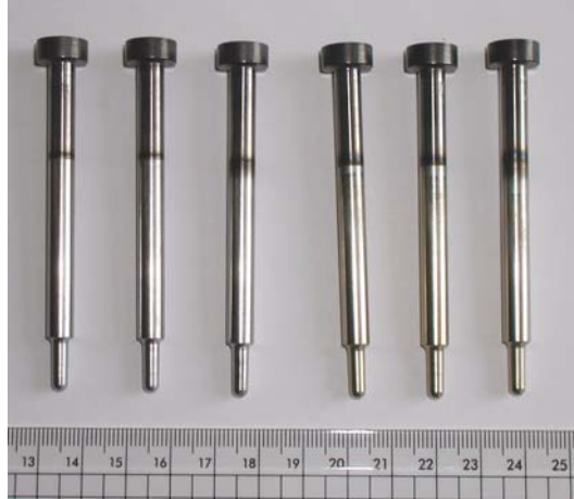
Figure 72: Ejectors coated with (W, Ti)C_{1-x} layer (3 Off on the left side) and with nc-Ti 2 N/nc-TiN nanocomposite layer (3 Off on the right side)
