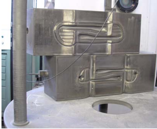
Figure 54: Die "FAF" after plasma nitriding
