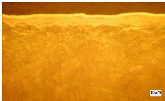
Figure 23: The compound layer produced by plasma nitriding on laser dispersing area
