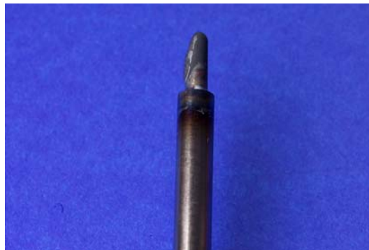
Figure 39: Deformation in the functional area after laser treatment – Ejector pins "DMF"
