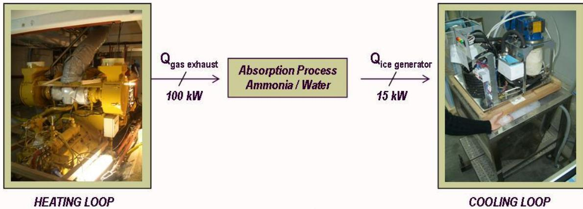
Once the thermal energy as well as the cooling load was determined, the design of the main parts of the IceMaker prototype started:
