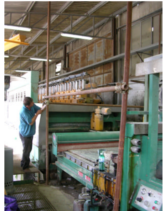
Figure 1 and 2: WOODSTONE metal structure positioned at the end of the traditional polishing work cycle
