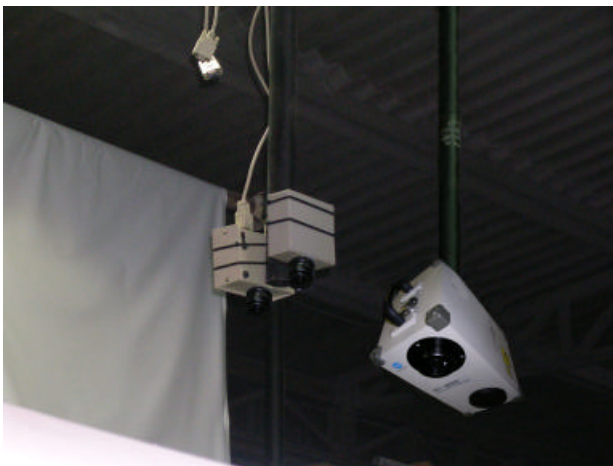
Figure 5 and 6: Details of the project equipment (camera, 3D scanner and hyperspectral system) positioned at the top of the WOODSTONE metal structure
