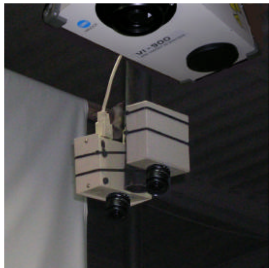
Figure 5 and 6: Details of the project equipment (camera, 3D scanner and hyperspectral system) positioned at the top of the WOODSTONE metal structure
