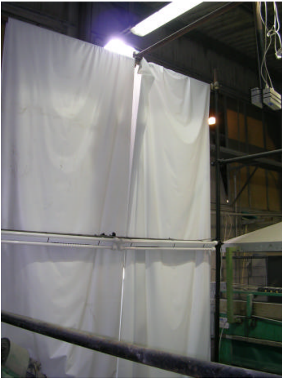
Figure 3 and 4: Details of the white sheets and of the neons positioned on the WOODSTONE metal structure
