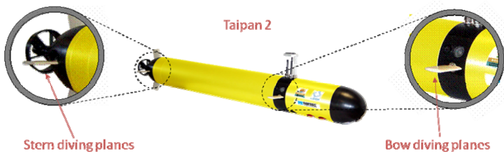
Figure 49: the full diving actuation of the AUV Taipan 2.
