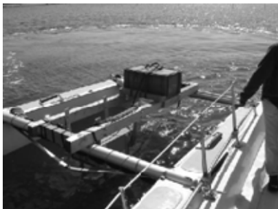
Figure 7: The catamaran structure for validation of the sensor suite. ©LIRMM-HYTEC
