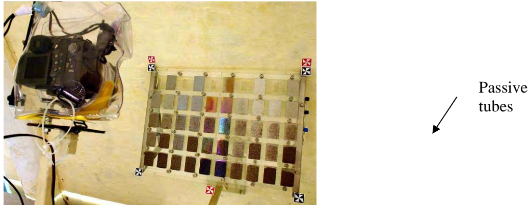
Figure 25 Shooting of the coupons on the rack at the beginning of the exposure period, Palace Armoury, Valletta. Note the presence of the passive tubes on the right of the rack for pollutants analysis.
