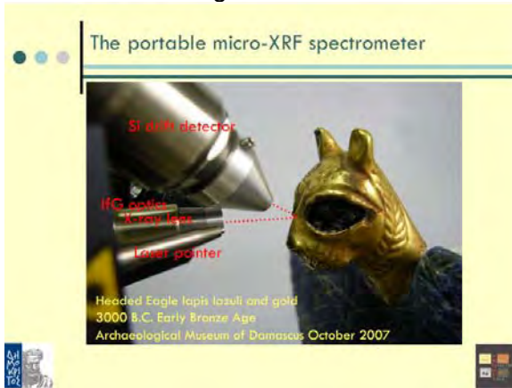
Photo of the micro-XRF measuring probe, designed and customized for Demokritos specifications (“open’ geometry), including the X-ray lens with 2 cm focal distance, a silicon drift detector and a ccd color camera for visual inspection of the analysis spot supported by a laser pointer.
