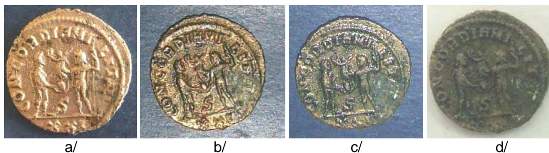
Figure 60 Coin 1 after FPTS application (a) and 10 days (b), 18 days (c) and 26 days (d) of exposure in the exhibition room of Umm Qais museum.
