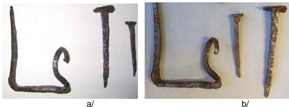
Figure 51 Condition state of three iron objects excavated from El Saucedo . (a) before application of Poligen ES 91009®. (b): after application and natural ageing (six months) in one of the laboratories of the UAM.
