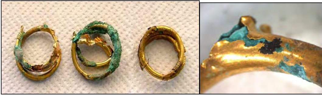
Figure 3 (left) Optical micrograph of gold-plated brooches for braid of hair with the enlargement of a cracked area of the brooch on the left (right)
