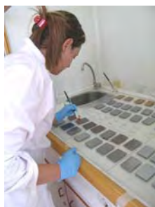
Figure 23 Application of Poligen ES 91009® on the steel coupons by brushing.
