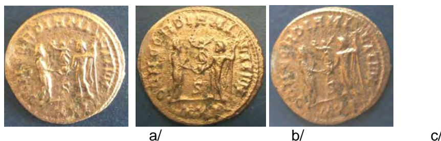
Figure 62 Coin 3 after silane A application (a), after three days (b) and five months (c) of exposure at Umm Qais museum (in the exhibition room).
