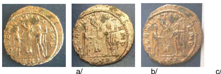
Figure 62 Coin 3 after silane A application (a), after three days (b) and five months (c) of exposure at Umm Qais museum (in the exhibition room).
