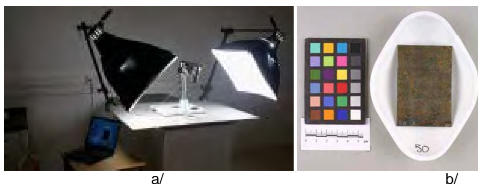
Figure 15 (a) Standard photographic documentation equipment; (b) coupon photographed under standard reproducible light conditions. Coupons were placed in “weighing boats” to facilitate their handling and prevent touching them during the whole ageing process.
