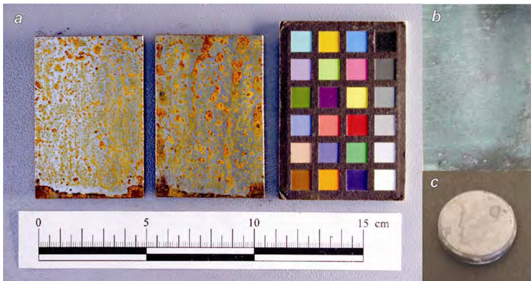
Figure 6 a) Steel coupons, prepared by HM/DMME b) Bronze coupons, prepared by SVUOM c) silver coupons.
