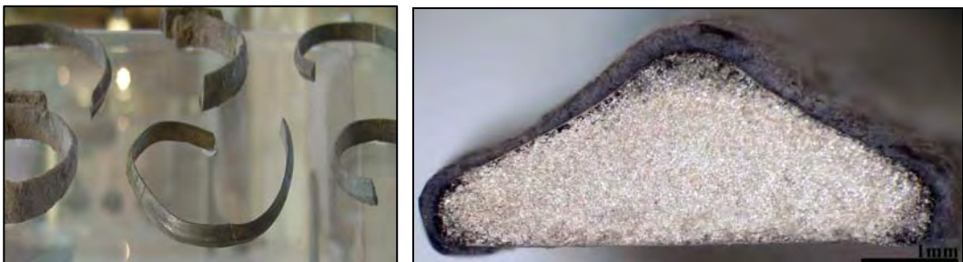
Figure 4 Carthaginian silver bracelets (left), optical images of the cross-section of a fragment (right)
