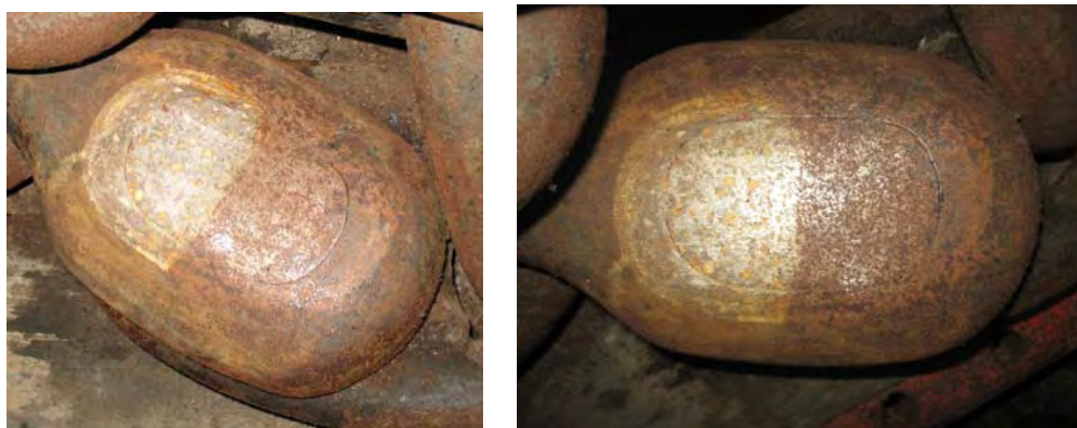
Figure 43 Corrosion progress on the chain element surface after 1.5 (left) and 9 months (right) of exposure in the storage area of the Maritime museum of Romainville Fortress.
