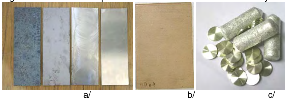
Figure 4 Raw material to produce steel coupons (from left to right: cast, sand blasted, milled and grinded) (a); (b) Quaternary bronze, grinded and polished; and (c) silver coupons (cast material and coupons after mechanical and heat treatment).
