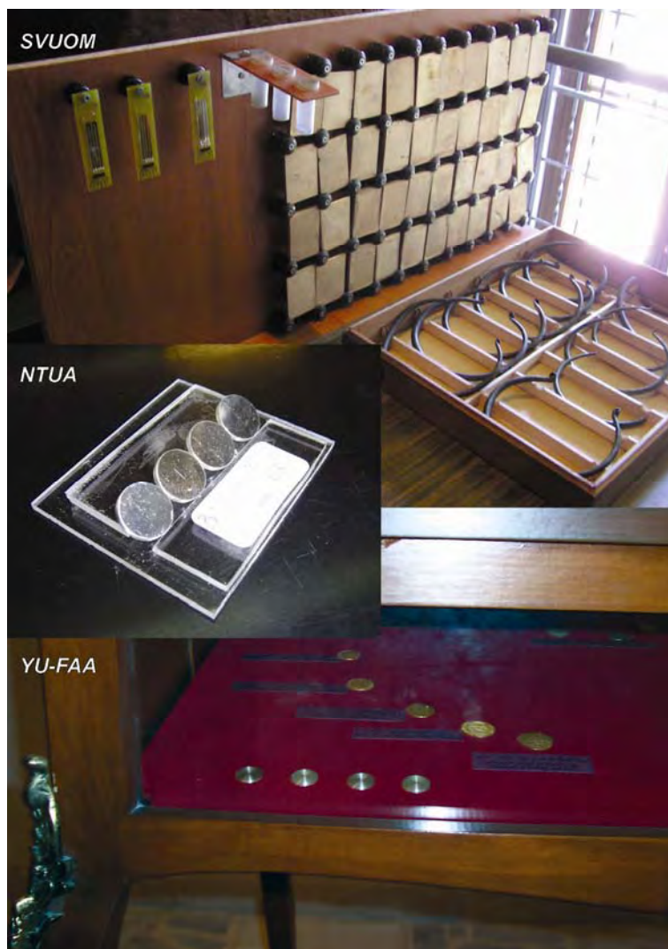
Figure 9 Overview of some of the conditions of exposure of the coupons (steel, bronze and silver-based) proposed by the partners.
