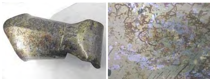
Figure 36 Condition state of one of the three fake gauntlets of the Palace Armoury, Valletta before intervention. Filiform corrosion developed under the polyurethane varnish.
