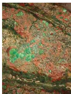
Figure 54 (a) Corrosion outbursts observed on the gilded horse tack protected with Poligen ES 91009®; (b) active corrosion observed on the bronze hook.
