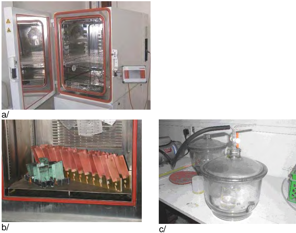
Figure 14 Accelerating ageing for the short-term testing of the protection systems on artificially aged coupons; (a) climatic chamber (TEI testing); (b) inside of a climatic chamber with copper plates and PROMET bronze artificially aged coupons (SVUOM testing); (c) stimulation of corrosion of silver-based coupons by exposure to a sulphide saturated atmosphere (80% ammonium sulphide solution, T= room temperature during 30 days) (YU-FAA testing).
