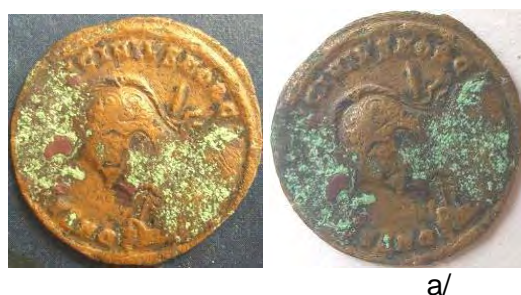
Figure 59 Back side of the unprotected coin before (a) and after the five months of exposure (b).
