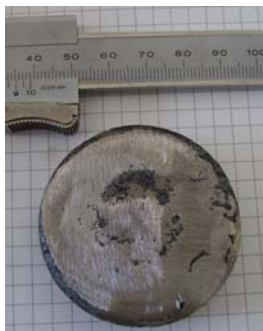
Figure 2. Fabricated ingots of the new material, which were aimed to be used for the final application (POLITO).
