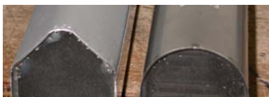
Figure 11. Prototypes of the second evolution stage atmospheric burner, with triangular and semi-circular mantel shape (BCT).
