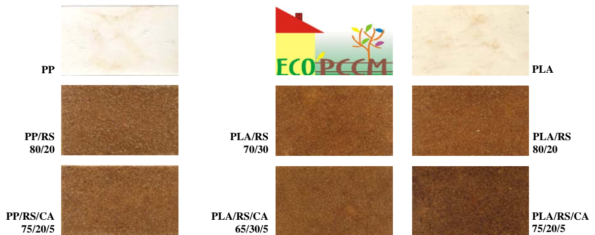
Figure 8. PP/RS/CA and PLA/RS/CA composites
