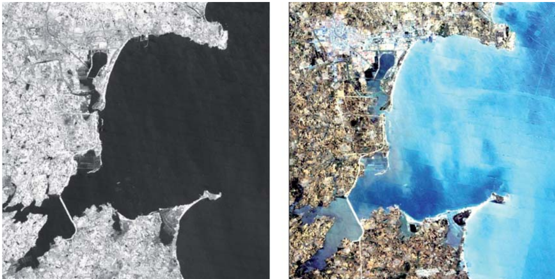
◆ FIGURE 36. Landsat scenes for Sanggou Bay used to determine regions of aquaculture. (Left) Band 5, near-IR, helps identify coastal features and fish cages. (Right) False colour scene picks out kelp structures.
