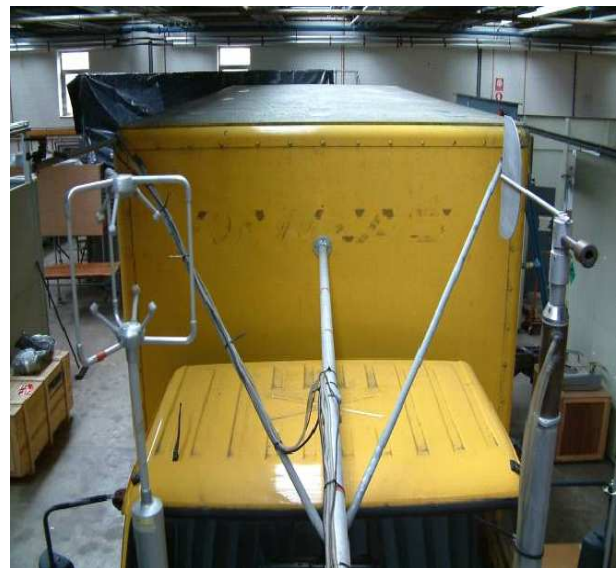
Figure 30 Front view. Front taps, anemometer
