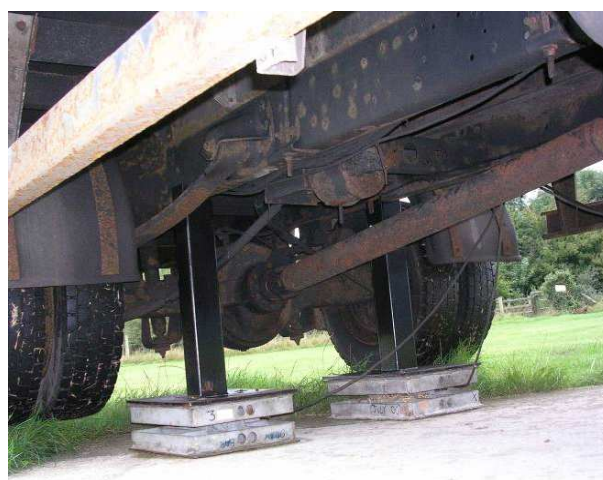
Figure 25 Load cells and steel support posts on the rear of the vehicle
