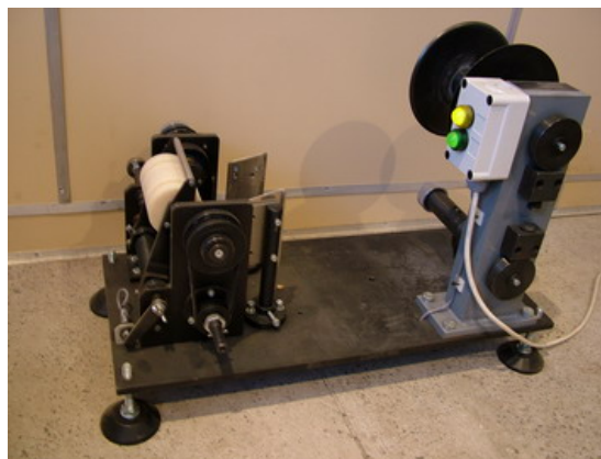
Figure 17: Machine for catalytic unit mechanical assembling
