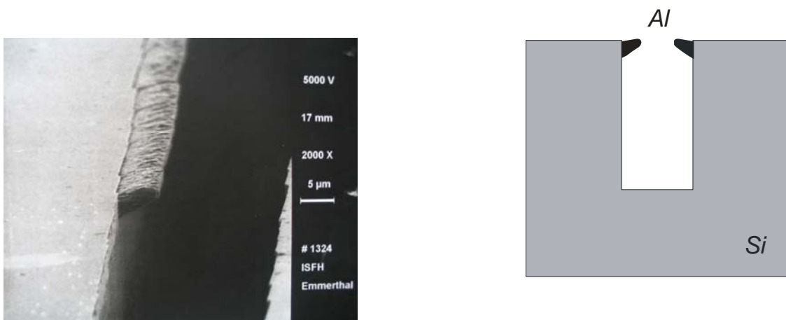
Figure 40: Aluminium contacts self-formation by oblique evaporation (ISFH)
