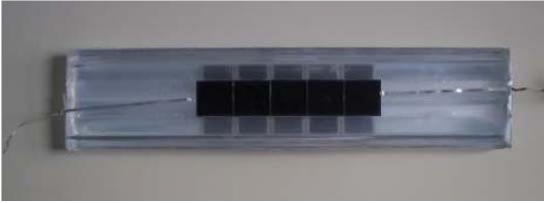
Figure 65: The solar-cell submodule with acrylic reflector provided by ISFH to CRES
