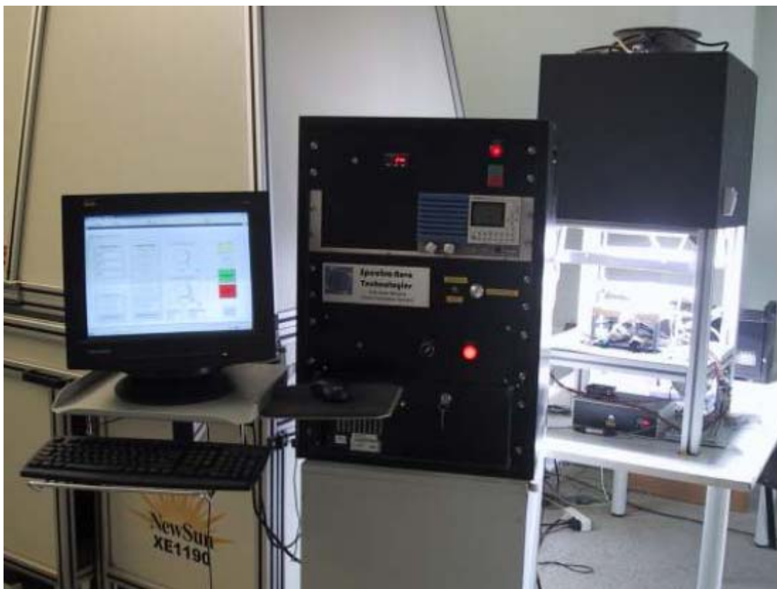
Figure 62: View of the solar cell tester at CRES PV laboratory
