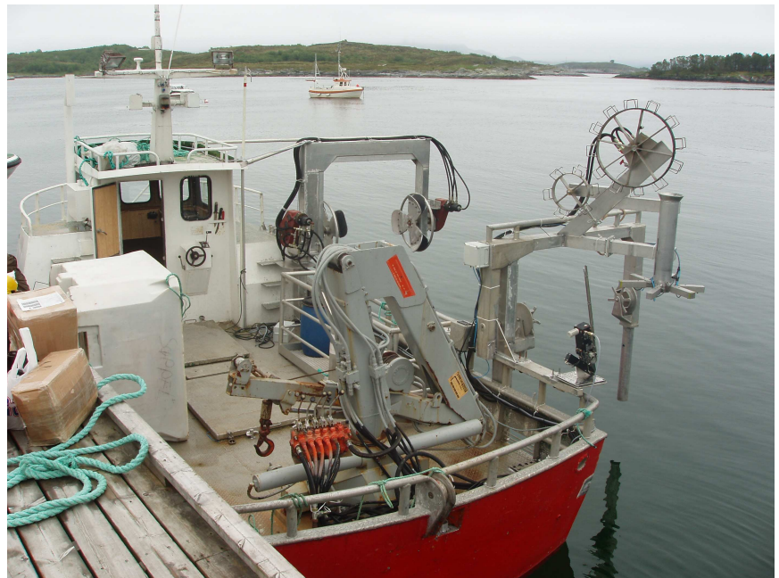
Mechanized system for attachment of mussel collectors and retubed mussel socks to longline, with integrated automatic sinker release unit.
