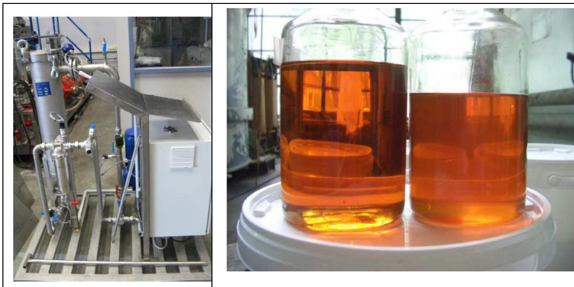
Figure 3. Moisture removal unit with conditioned (left) and contaminated (right) oil samples
