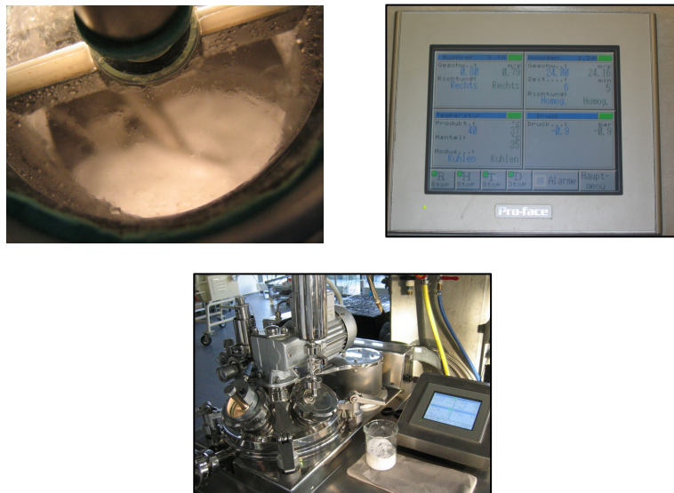
Figures 22, 23 and 24: Mixer at different steps on the production: mixture, cooling down and homogenisation
