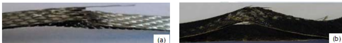
Figure 28: Failed (a) carbon fibre reinforced and (b) glass fibre reinforced Biorez samples
