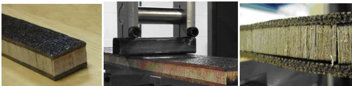
Figure 24: Sandwich panel Failure type and locus for the furan/balsa sandwich
