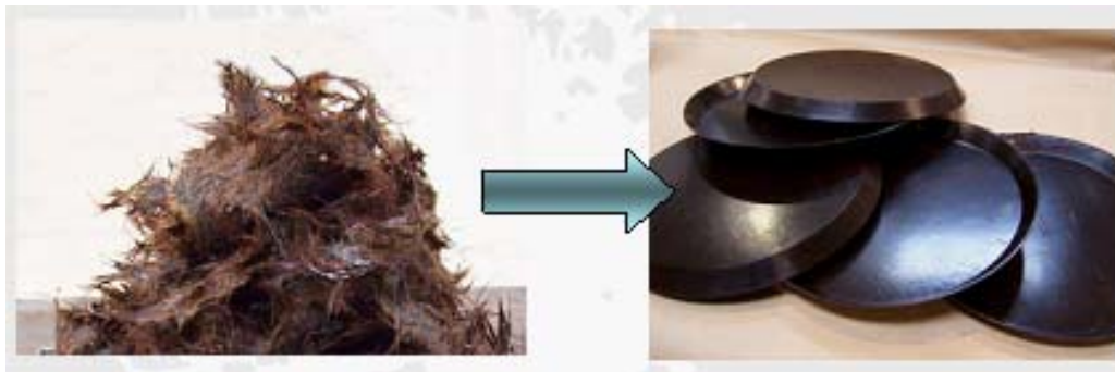
Figure 25: BMC processed to trays by hot compression
