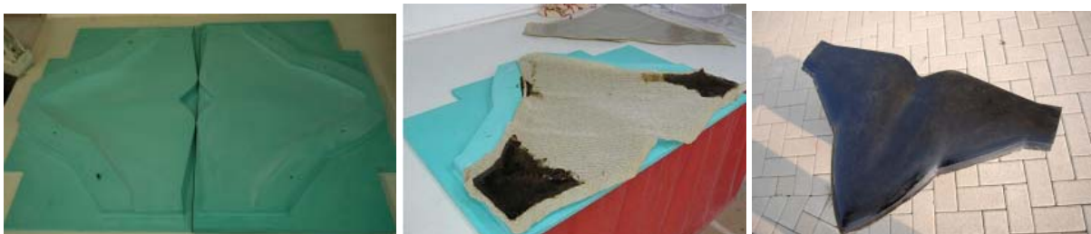
Figure 27: Processing the natural fiber reinforced Mini UAV
