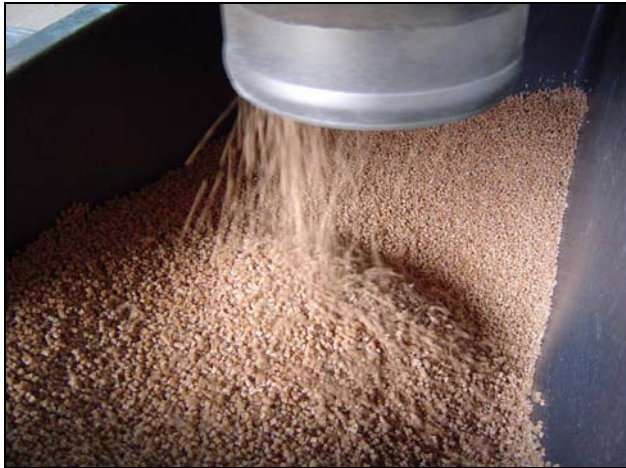
Figure 16: Compounds manufactured by the planet screw extruder
