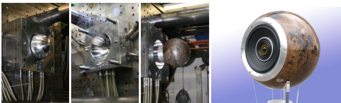
Figure 8: Mould for a spherical loudspeaker cover with wall thickness of 10mm and a diameter of 250mm and the surface finished completed box
