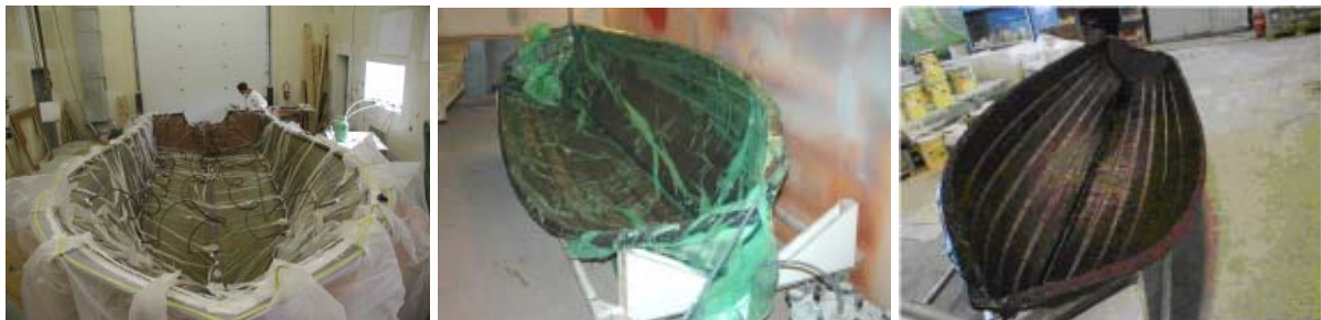
Figure 23: vacuum infusion to manufacture a boat
