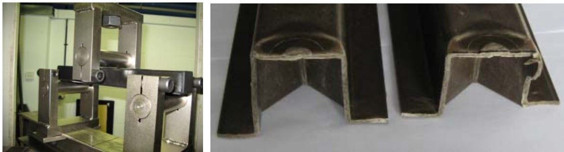
Figure 13: Bending tests and broken beam
