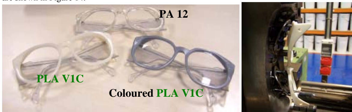
Figure 14: Eye glasses frames in comparison of an impact modified PLA with PA 12 and a testing equipment
