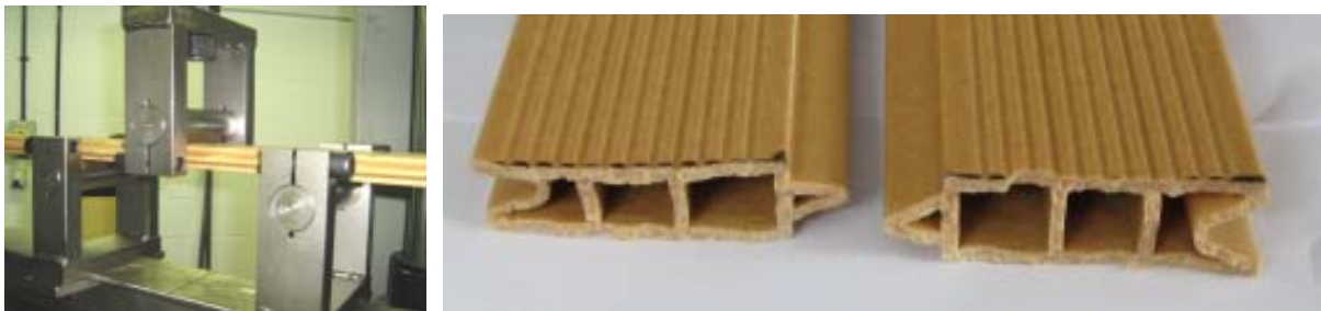
Figure 17: Bending test of extruded beams from PLA and natural fibers
