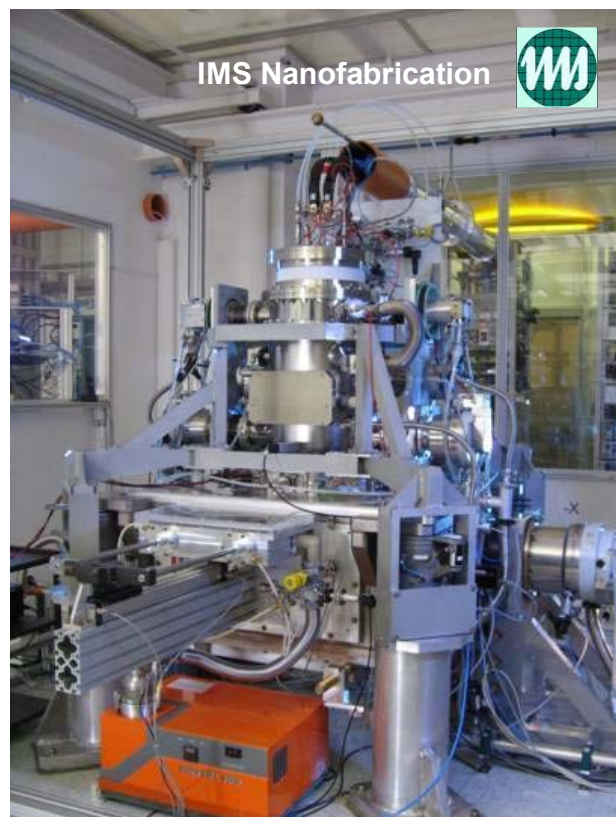
Figure 1: Principles of Charged Particle Nanopatterning and realized CHARPAN Prototype Tool
