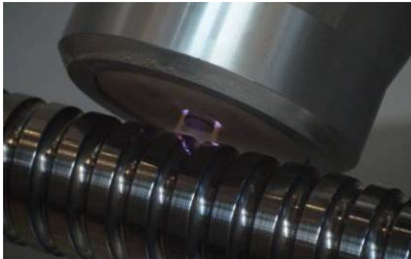
Figure 19: Coating of the Fatronik demonstrator with atmospheric plasma torch (VITO)
