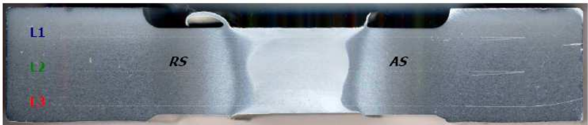
Figure 4.13: Hardness profiles on 4 coupons (average of 3 line measurements on each coupon). Beneficial effect of a T79 post welding heat treatment Picture of the measurement lines on the coupons.
