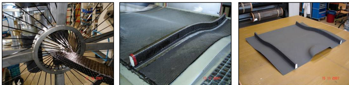
Figure 14: Manufacturing steps for the EADS-G validation example
