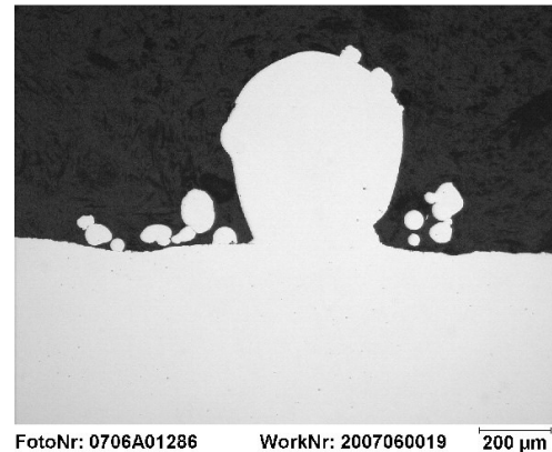
Figure 1: Cross section of a laser cladded structure.
