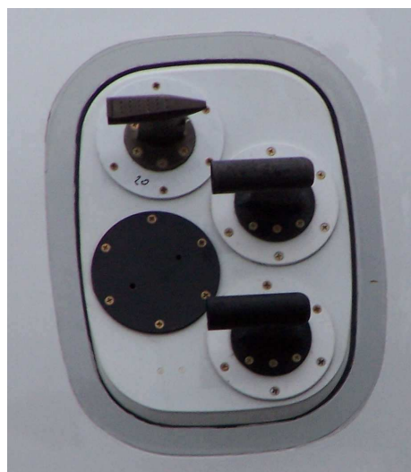
Figure 40 : DETAIL OF THE WINDOW FOR THE STATIC PORT AND THE MATERIAL PROBES
