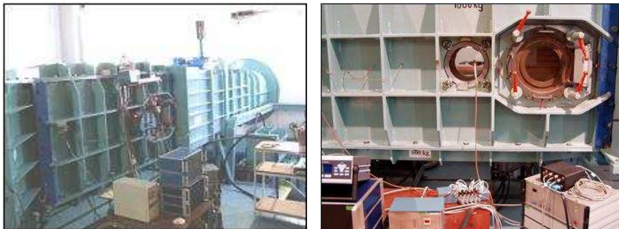
Figure 8 : Pictures of the Transonic Wind tunnel at VZLU
