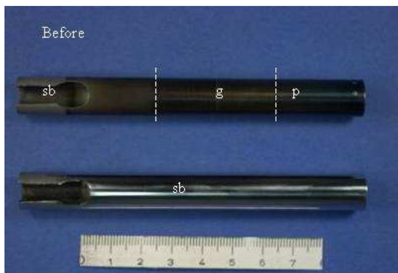
Figure 15 : Aspect of the tube before test (sb=sand-blasted, g=grinded, p=polished)
