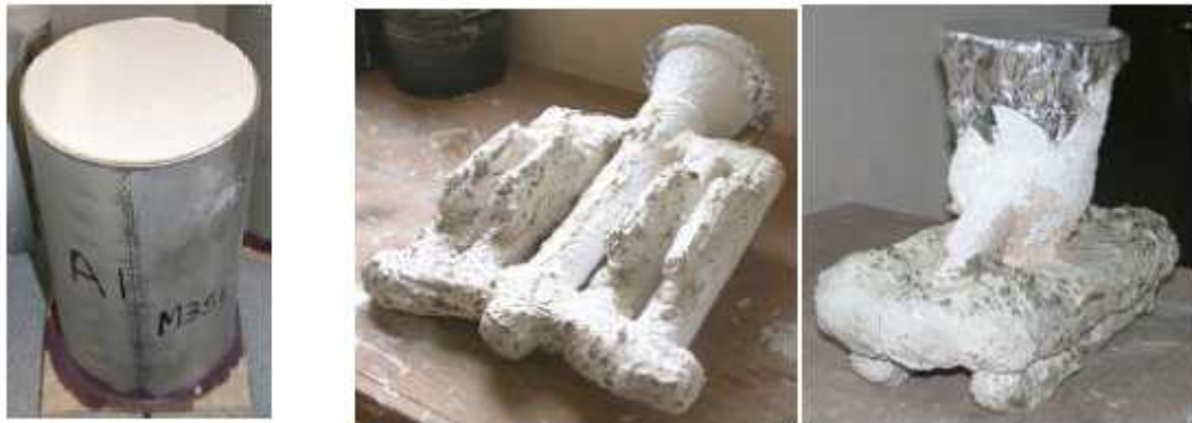
Figure 10 : Plaster mould for aluminium (left) and shell moulds for steel (right)
