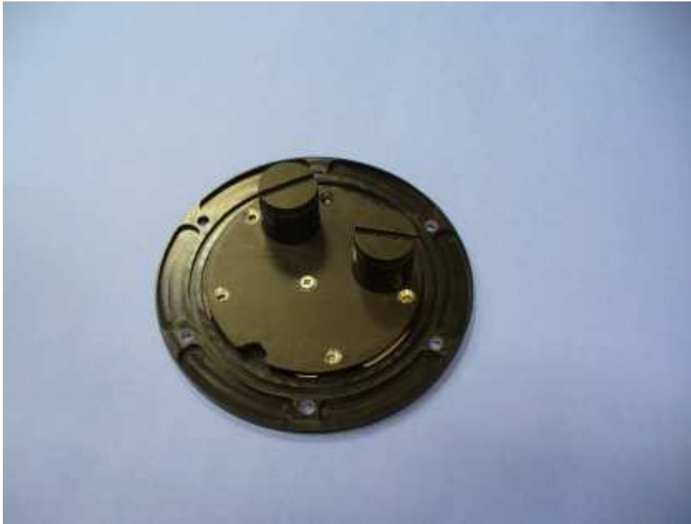
Figure 32 : mock-up of the heated static port
