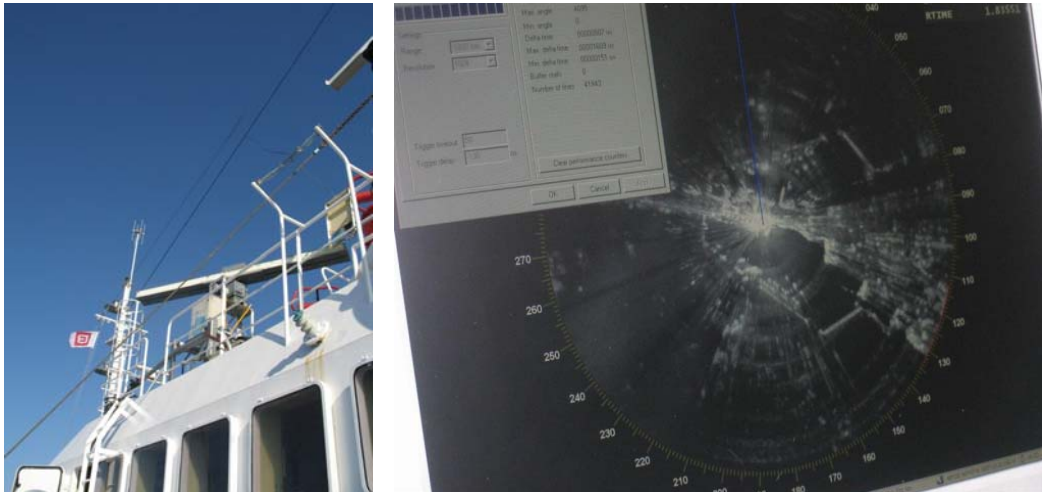
Very recent systems today allow getting real time wheelhouse information about the location of oil slicks around the vessel (which proves extremely difficult visually), using the bare signal from the radar (Here: the SeaDarq system tested at sea by Cedre and the French Navy)
