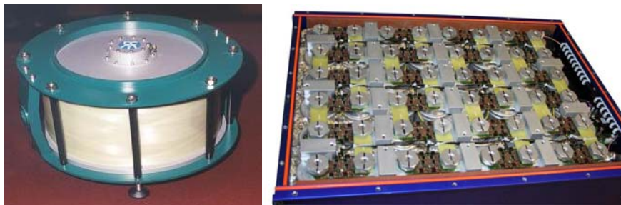
Figure 26: Different types of storage systems (left: Flywheel of CCM, right: Ultracapmodul)
