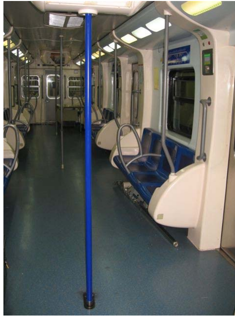
Figure 29: lightweight grab rail on the Metro de Madrid MODURBAN demonstrator train.
