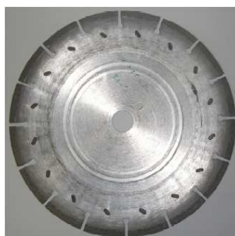
Figure 11 - Design of the first mart cutting disc prototype
