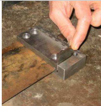
Figure 9 - Blade holder with SMAs inserts solution B
