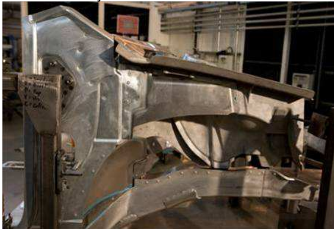
Figure 8: Front end lateral view with longitudinal front rail assembled by adhesive glue + self piercing riveting , inner A pillar reinforcement and upper long front member assembled by adhesive glue + self piercing riveting
