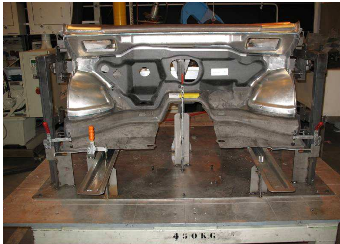
Figure 9: Front end rear view with hot press steel rocker transversal beam assembled by CMT weld brazing, water boxes assembled by adhesive glue + self piercing riveting, Carbon Fiber Reinforced Composite mounting plate joined by adhesive glue.
