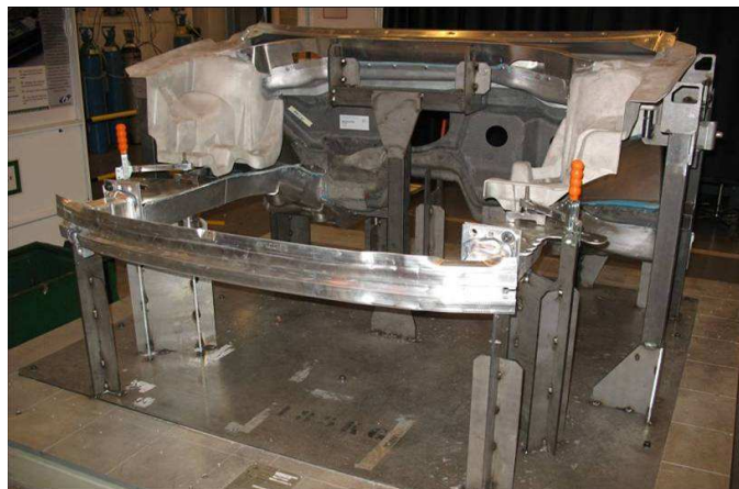
Figure 6: Front end front view with aluminum bumper assembled by MIG welding, magnesium strut tower assembled by adhesive glue and screwing
