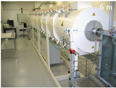
Figure 44 - Photograph of a long (6 m) tubular furnace with controlled atmosphere and 16 zones of temperature control. Buffer layer growth and YBCO pyrolysis can be performed in this furnace.
