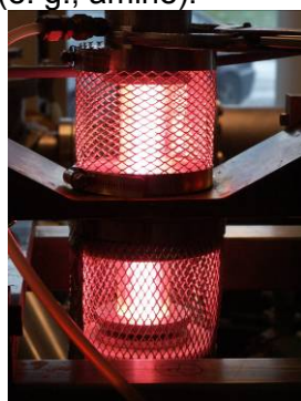
Micro wave-assisted cold plasma technique. device used at UMH
