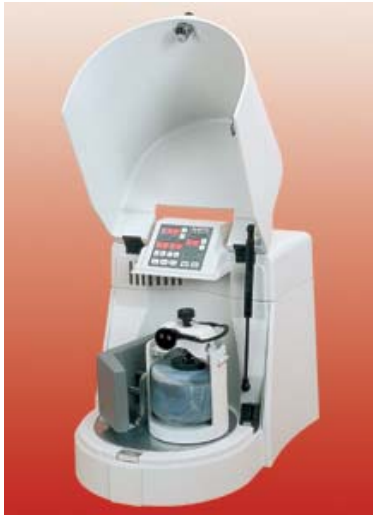
Fig. .2 Ball mill for quick and simple tests of mechanical stability (ZSW).
