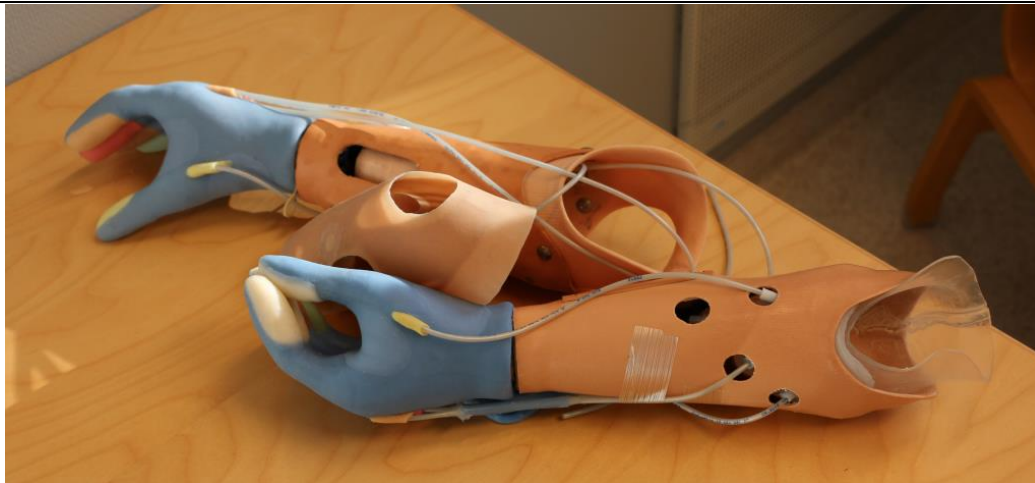
Figure 3: The custom liner with the integrated actuators, the fitted socket and the hand prosthesis with force sensors.
