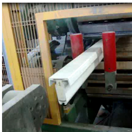
Figure 9. Final industrial profile. PVC glass fiber reinforced, PS foamed inside.
